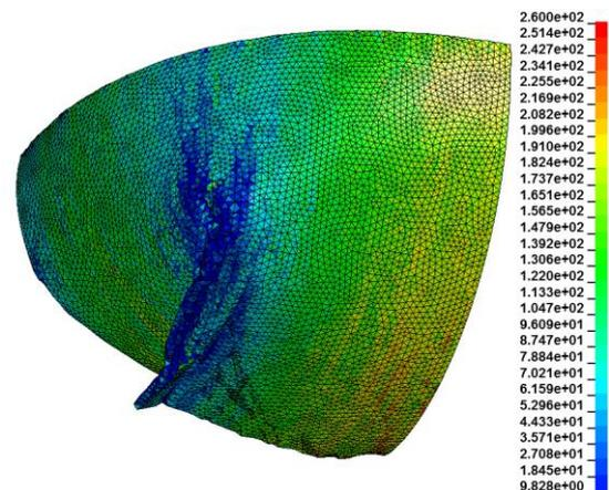
Figure 5: Calculated stresses in X-direction (longitudinal)
