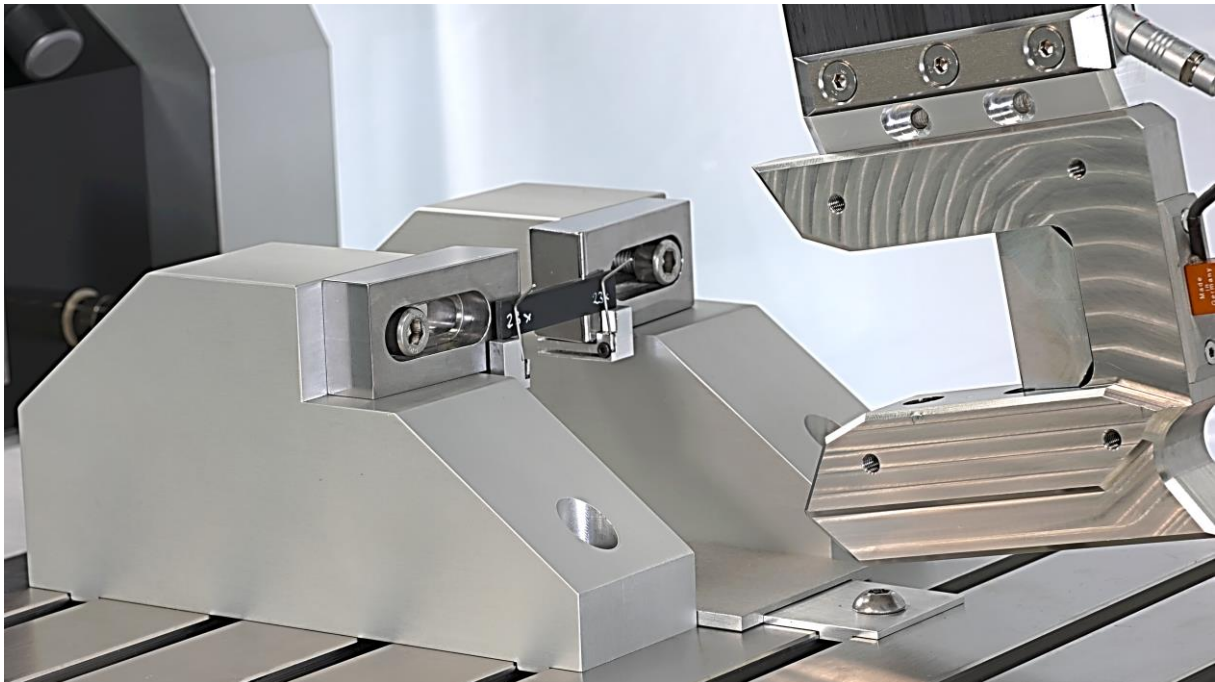
Figure 19: Test setup dynamic 3PB
