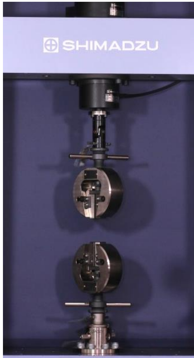
Figure 27: Shimadzu AG-X tensile test setup
