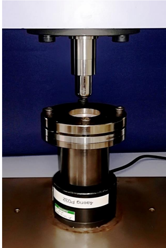
Figure 36: Static puncture test setup
