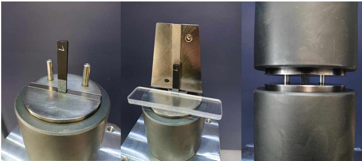
Figure 53: Clamping the Celanese specimen
