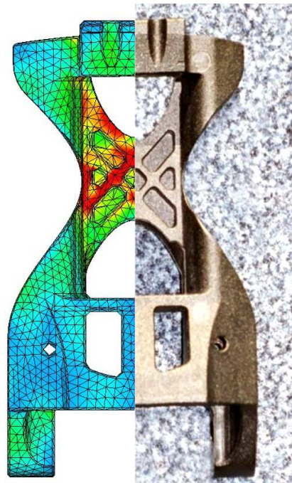
Fig.: From virtual structural simulation of the 3d geometry to the real part.
